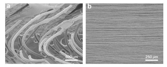
**Figure S3**. SEM images of the middle part of a pressed TET (a) and aligned carbon nanotube (CNT) sheet (b).
