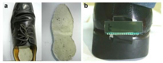
**Figure S11.** An insole made from a TET (a) and a LCD lightened by people walking (b).
