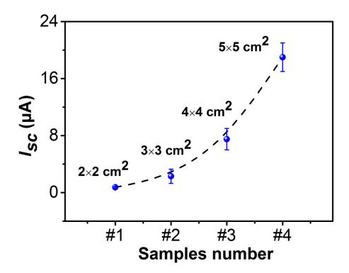
**Figure S5.** Dependence of short-circuit current on size of the TET with the same thickness of 8 mm at a pressing frequency of 1 Hz and force of 16 N per square centimeter.
