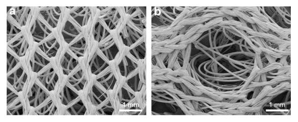
**Figure S2.** Scanning electron microscopy (SEM) images of the top (a) and bottom (b) surfaces of the fabric from poly (ethylene terephthalate) (PET) fibers.
