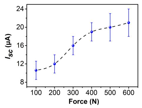
**Figure S7**. Dependence of short-circuit current on pressing force at a pressing frequency of 1 Hz for a TET with thickness of 8 mm and size of  $5 \times 5$  cm<sup>2</sup>.
