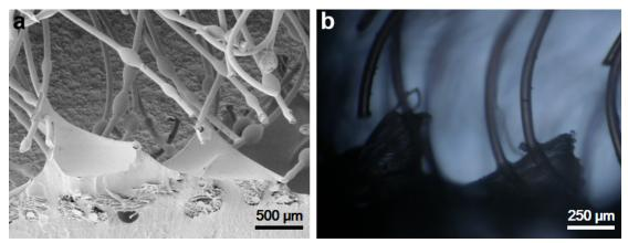
Figure S10. SEM image and optical micrograph of the PDMS pyramids.
