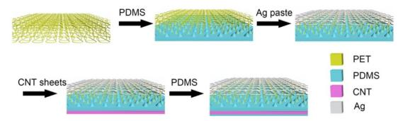
Figure S1. Fabrication process of the triboelectric textile (TET).
