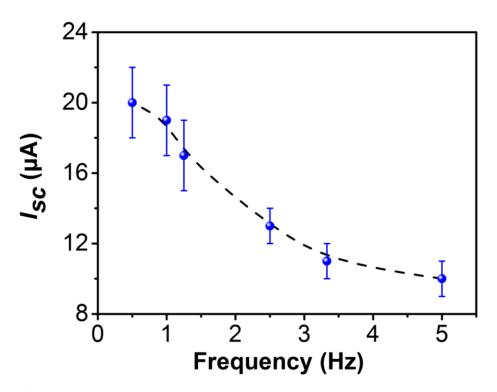
**Figure S6**. Dependence of short-circuit current on pressing frequency at a pressing force of 400 N for a TET with thickness of 8 mm and size of  $5 \times 5$  cm<sup>2</sup>.
