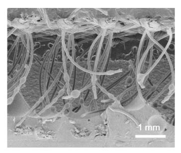
Figure S8. SEM image of a TET after pressing for over 3000 cycles.
