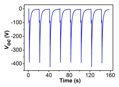
**Figure S4**. Open-circuit voltage of a TET where the output voltage returned to 0. The TET showed a thickness of 8 mm and size of  $5 \times 5$  cm<sup>2</sup>.
