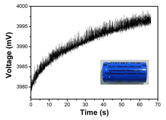
**Figure S12.** The charging curves of a lithium ion battery with a capacity of 1200 mAh by pressing a TET (inset, photograph of the lithium ion battery).
